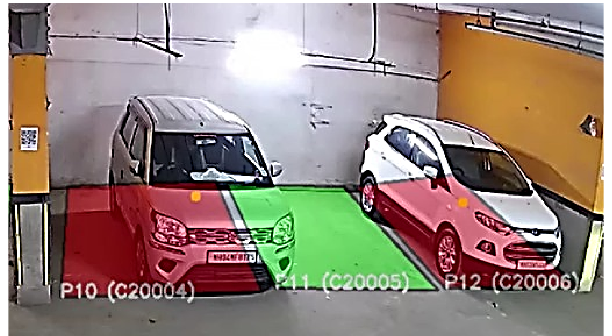
Smart detection of mis-parked vehicles & vehicle presence per slot
